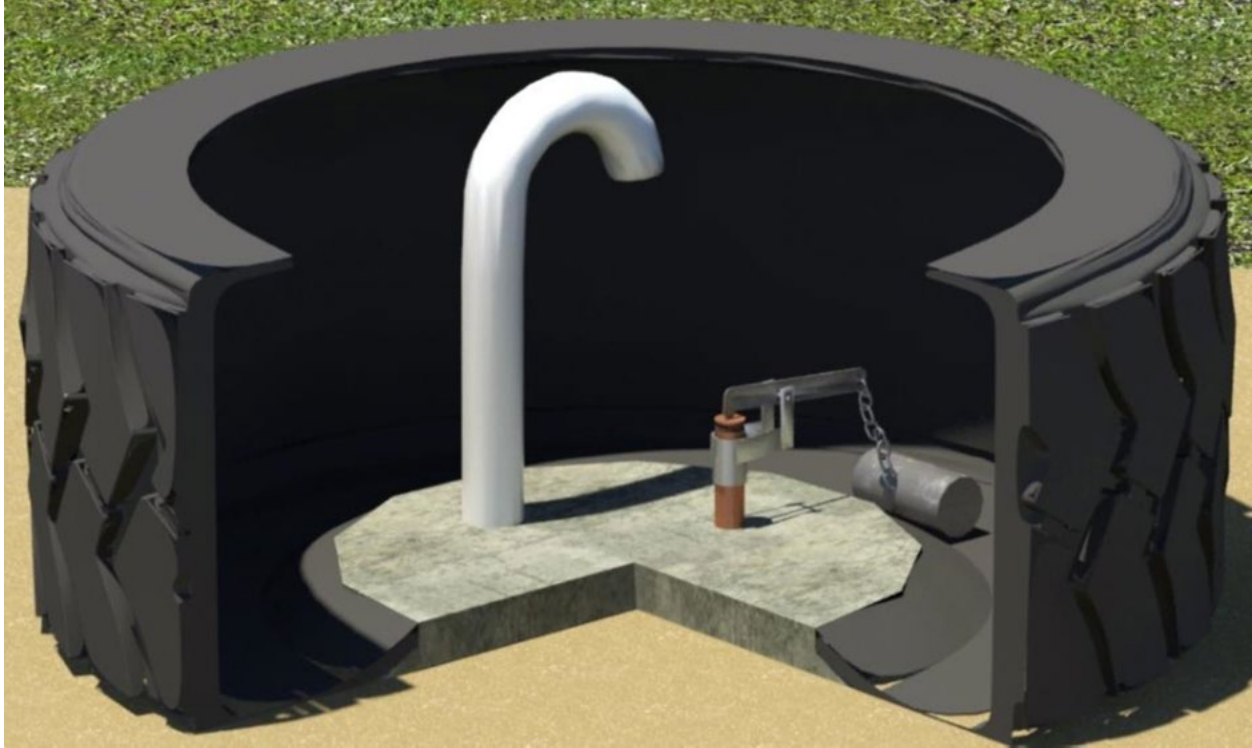
Figure 3. A cross-section of a tire waterer.
