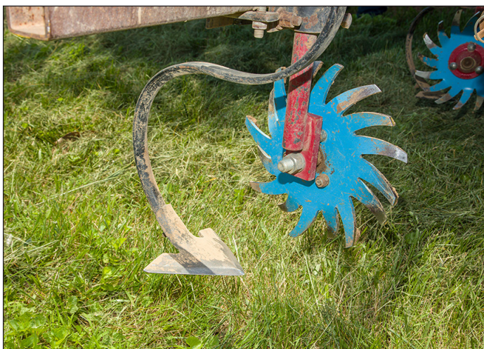
A COMBINATION OF DANISH S-TINES AND SPYDERS THAT ARE USED TO CULTIVATE BETWEEN ROWS.
