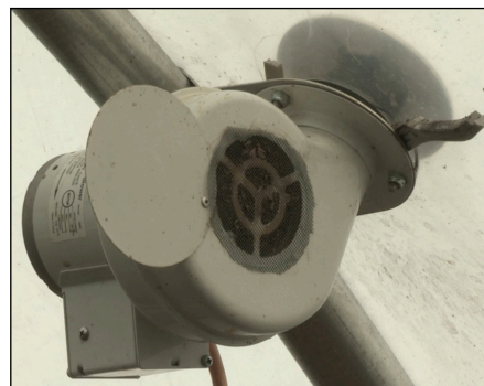
An inflation fan creates a layer of air between two layers of plastic, which provides more protection from cold weather in a high tunnel.
