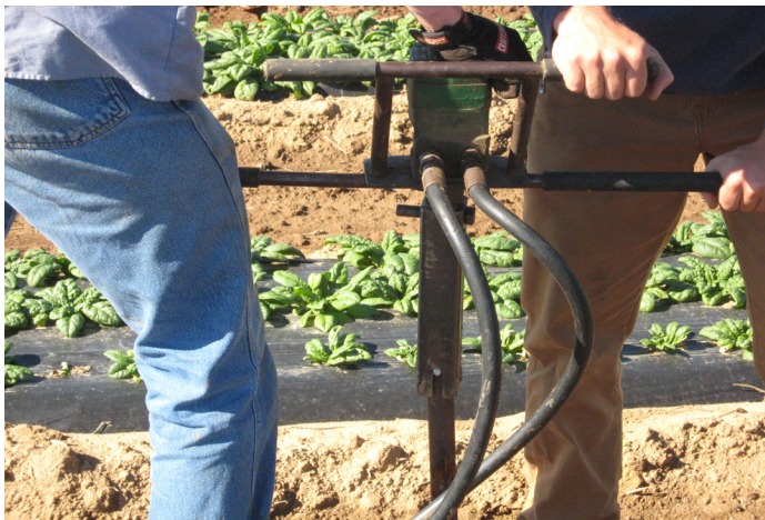
A hydraulic-driven tool that drives anchors into the ground and helps remove them can make anchoring easier. You will need the tool and a tractor to power it. Photo: Tim Coolong
